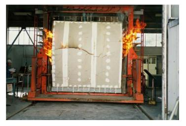
These systems can provide fire ratings of up to 2 hours to meet the BCA requirements for various types of construction. For more information see the James Hardie Fire & Acoustically Rated Walls technical literature.
